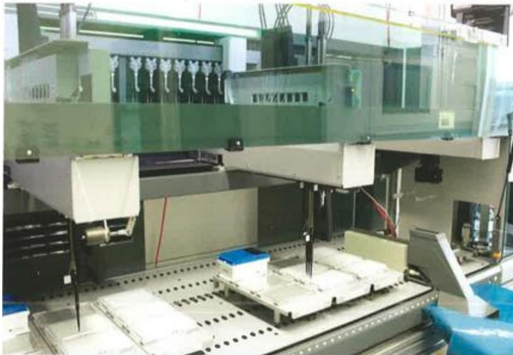
Automation on a Freedom EVO platform enables cost-effective, high throughput HLA typing
